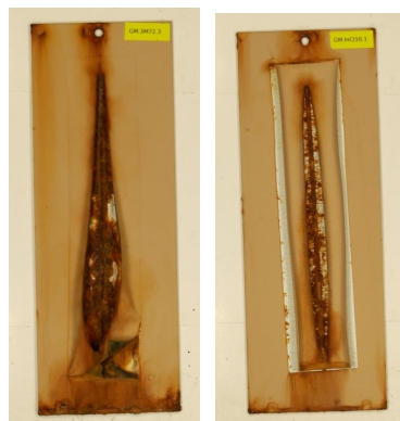
Scribed Appliqué Delamination Both panels show appliqué material delaminating from epoxy layer
