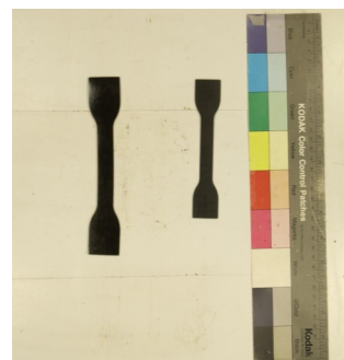
Figure 2. Photo showing swelled rubber (left) versus unexposed material (right).
