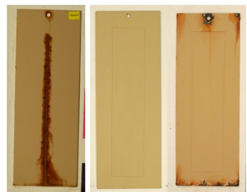
Repaired Panels Corroded panel before repair (left), Repaired panel with appliqué and CARC (middle), Destroyed repair panel (right)
